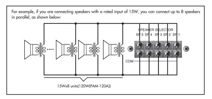
**WARNING:** Extreme care must be exercised when connecting low-impedance systems, as potentially hazardous voltages may be present at these terminals.
