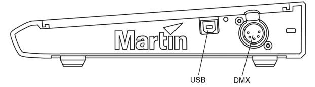
A USB-B 2.0 connector is placed on the right-hand side of the Martin<sup>™</sup> M-Touch for connection to a host PC. The M-Touch can draw a maximum of 500 mA. If you use a USB hub, make sure that it is powered.
